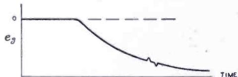
Fig. 11—Grid-voltage pattern when tube has recovered.
