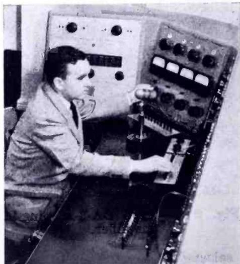
Fig. 7—Console operating position showing the monitor key-switches and microphone controls.
