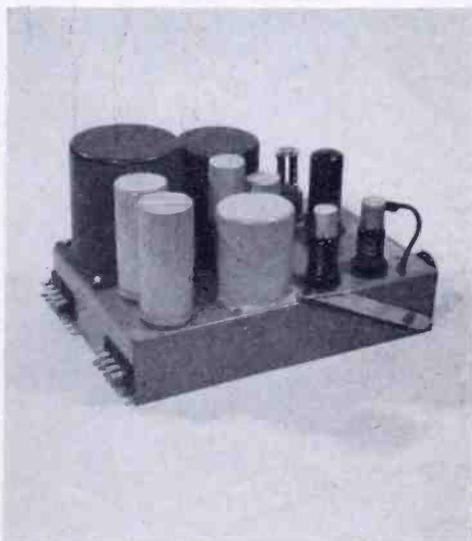
Fig. 6 — Type BA-3-A plug-in amplifier.
